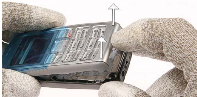
5.) Remove the A-Cover . Always start on the top side of the device when re-assembling the A-Cover.
