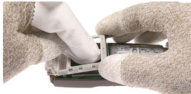
8.) Lift the LCD Shielding while pressing on the LCD Module with a clean cloth carefully.
