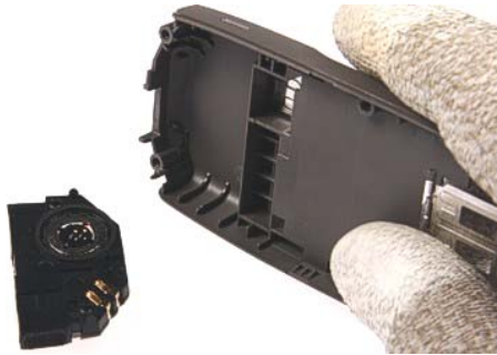
17.) The Antenna IHF Assy drops out when turning the D-Cover Assy .
