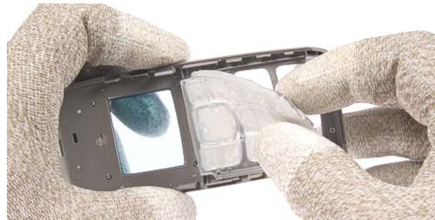
6.) Remove the Keymat and protect the inner side of the window with a film.
