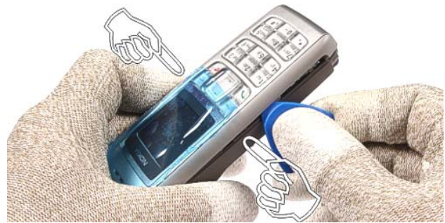
4.) Use the SRT-6 to unlock the A-Cover on both sides.
